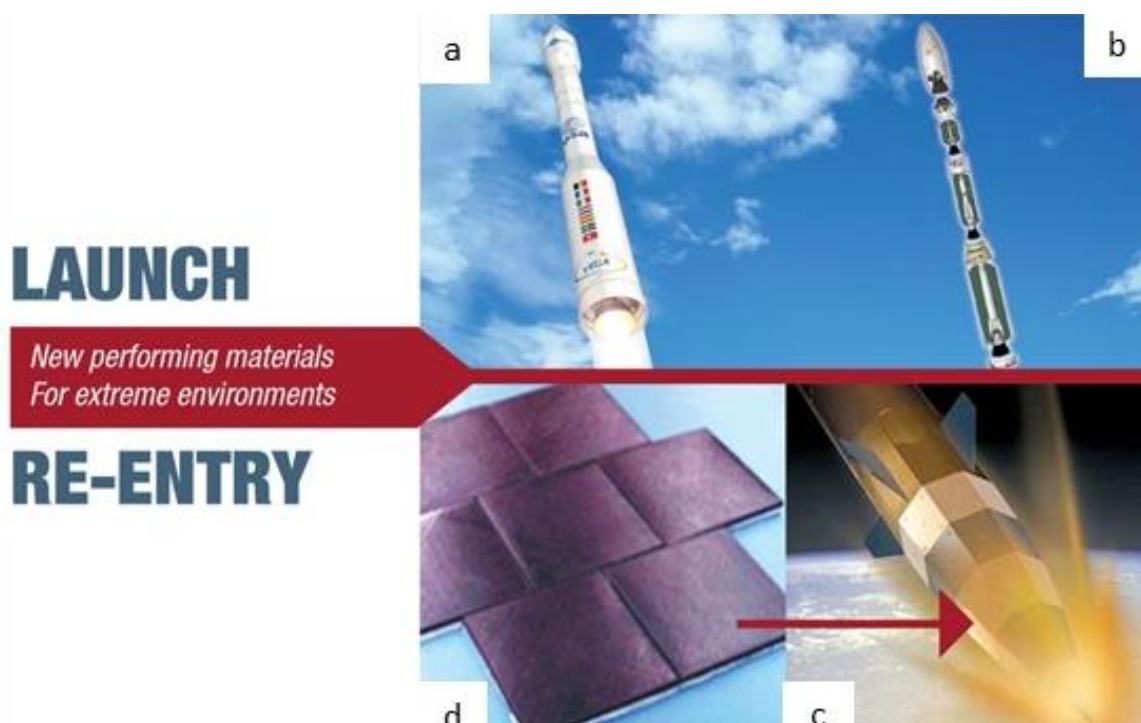
Figure 1 a) Vega launcher and b) sketch of the various stages of launch, indicating the position of nozzles for civil aerospace rockets c) SHEFEX I re-entry experiment (courtesy of DLR) d) CMCs tiles for thermal protection systems
