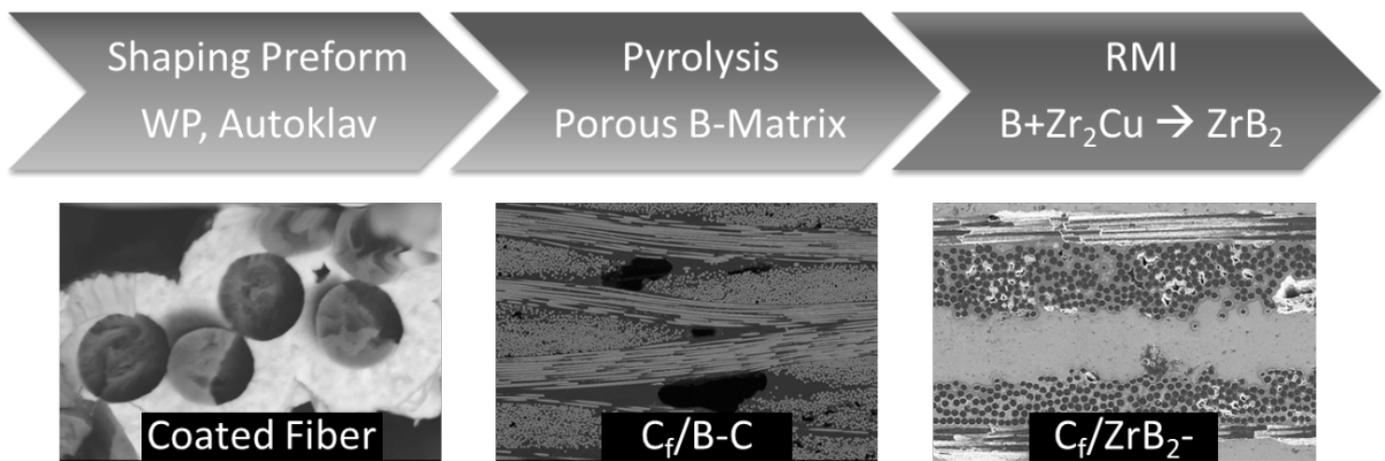
Figure 4: Schematic of RMI process.
