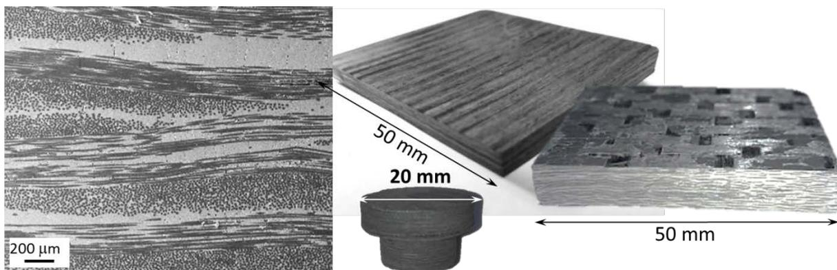
Figure 2: Microstructural features of pellets and small prototypes produced by HP and SPS.
