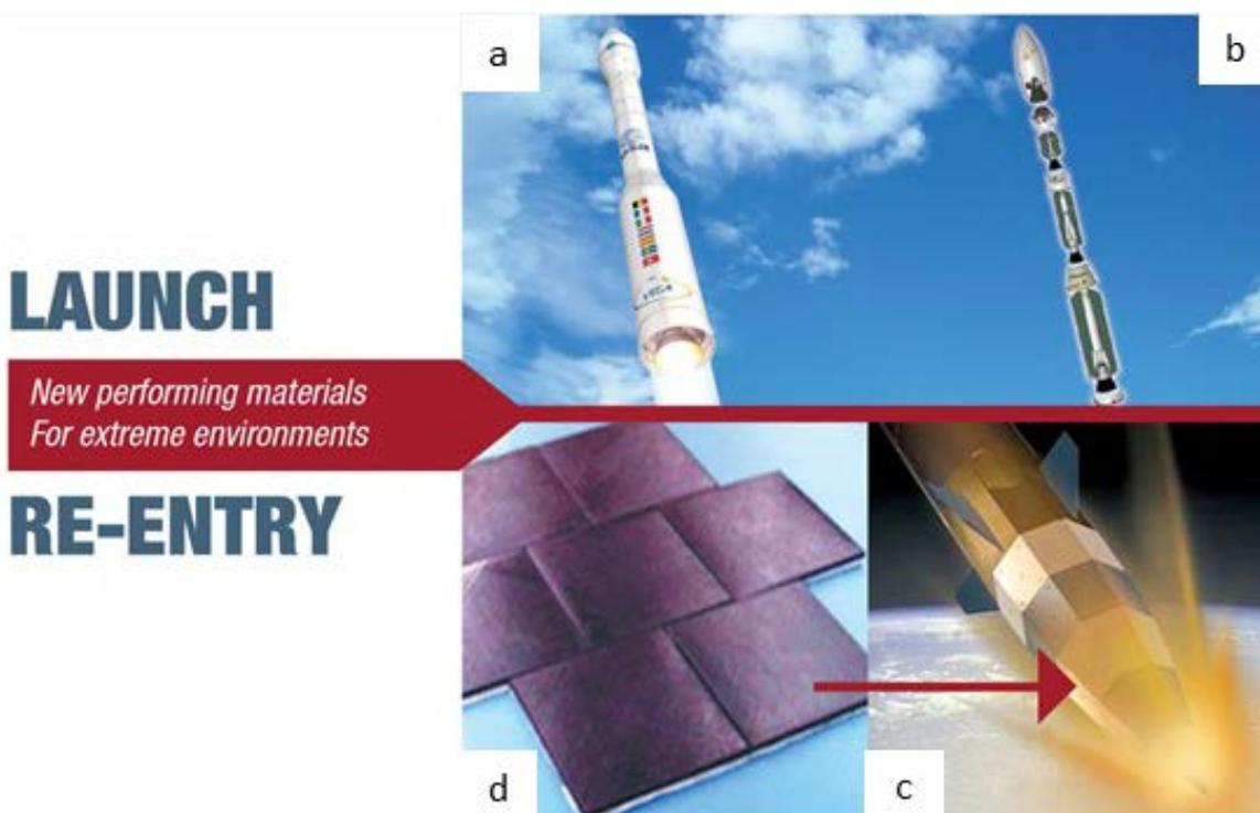
Figure 1: a) Vega launcher and b) sketch of the various stages of launch, indicating the position of nozzles for civil aerospace rockets c) SHEFEX I re-entry experiment (courtesy of DLR) d) CMC tiles for thermal protection systems.
