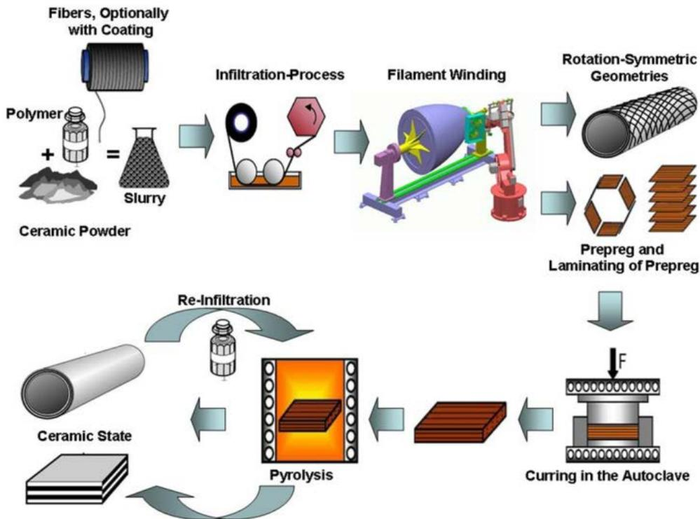
Figure 5: Polymer-Infiltration-Pyrolysis (PIP) process
