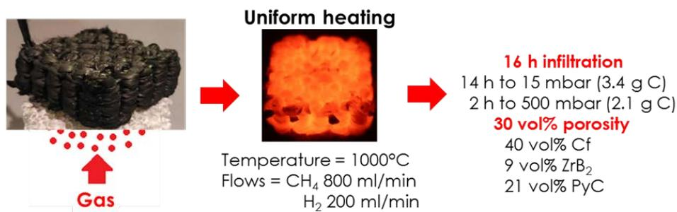
Figure 3: Illustrations of the preforms, heating and current densities achieved using RF-CVI of C matrix
